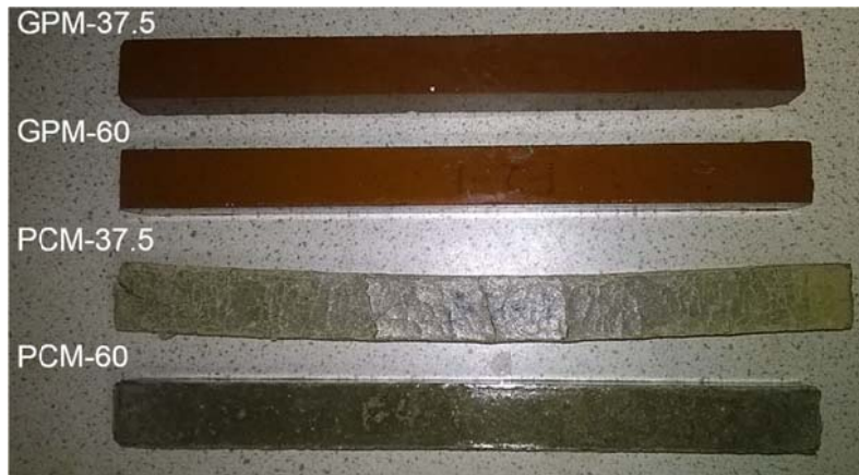
Figure 5 Samples of GPMs and PCMs after 32 weeks of exposure to Na 2 SO 4 solution
