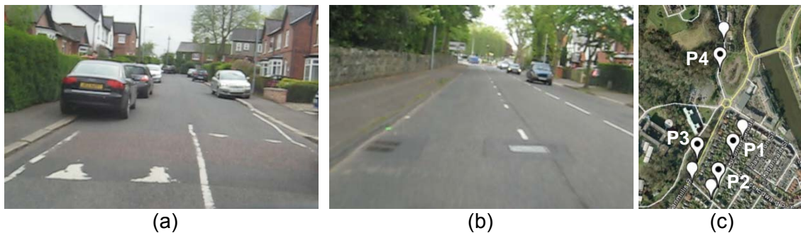
Figure 7: Video screenshots of peak locations (a) at P2 (b) at P3 and (c) Vehicle position coordinates identified (black dots) at peak locations using smartphone and Leica GNSS.
