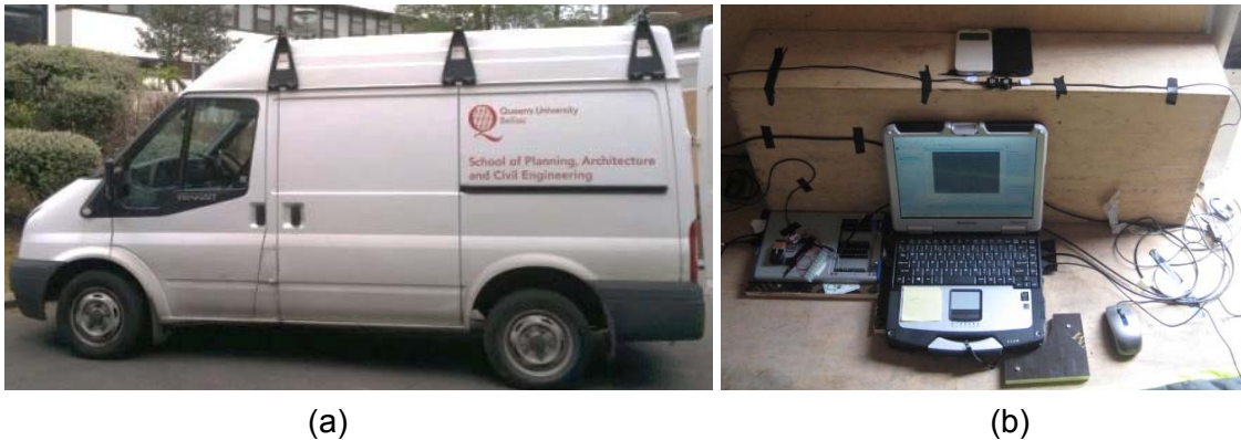
Figure 5: (a) Instrumented vehicle and (b) data acquisition system
