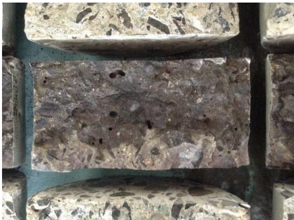
Figure 10 Splitting sample slices sprayed with Silver Nitrate
