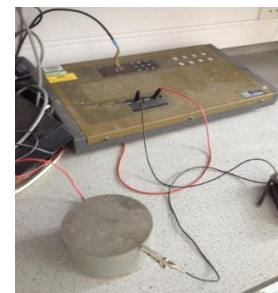
Figure 2 Bulk resistivity test equipment and sample
