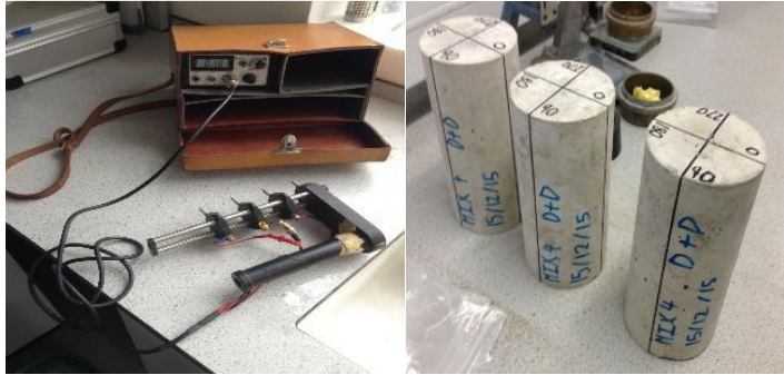
Figure 3 Surface resistivity test equipment and samples
