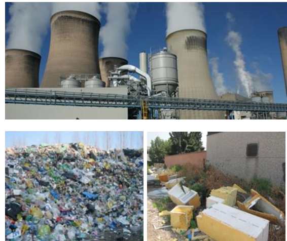
Figure 1. Secondary raw materials integrated in SUS-CON concretes: industrial by-products (PFA, GGBS) and post-consumer plastics (mixed plastics and rigid polyurethane foams) / Materie prime seconde utilizzate nei calcestruzzi SUS-CON: sottoprodotti industriali (PFA, GGBS) e plastiche post-consumo (plastica mista e schiume rigide di poliuretano).
