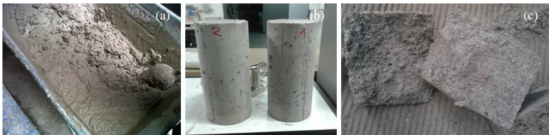
Figure 2 Fresh (a) and hardened concrete samples (b, c) based on RX and OPC.
