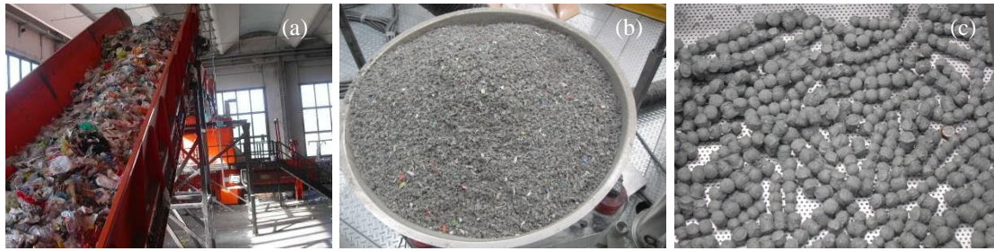
Figure 1 Mixed plastic scraps (a) used as raw materials for RX aggregates production: densified flakes (b) and expanded granules (c).
