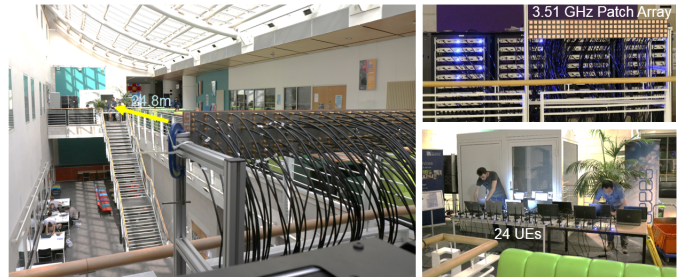
Fig. 2. Second measurement trial with the UEs 24.8m away
