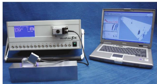
Figure 1: A commercial phased array controller, phased array, metal sample and imaging software. (Image courtesy of MicroPulse USA.)
