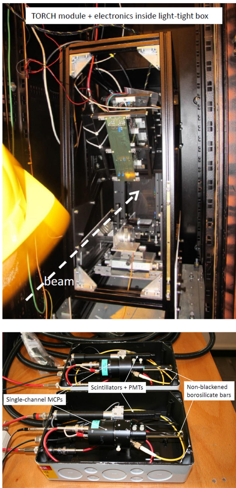
Fig. 7. (Top) The TORCH prototype module comprising a radiator plate of 120 \times 350 \times 10 \text{ mm}^3 , a focussing block, a Phase-2 MCP-PMT, and customised electronic boards. (Bottom) The scintillation finger modules and borosilicate bars with single-MCPs to provide a trigger and timing reference, respectively.
