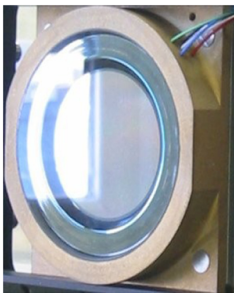
Fig. 2. (Left) View through the entrance window of the Phase-2 Photek MCP-PMT, which has an active area of 26.5 \times 26.5 \text{ mm}^2 ; (Right) The backplane of the MCP-PMT.
