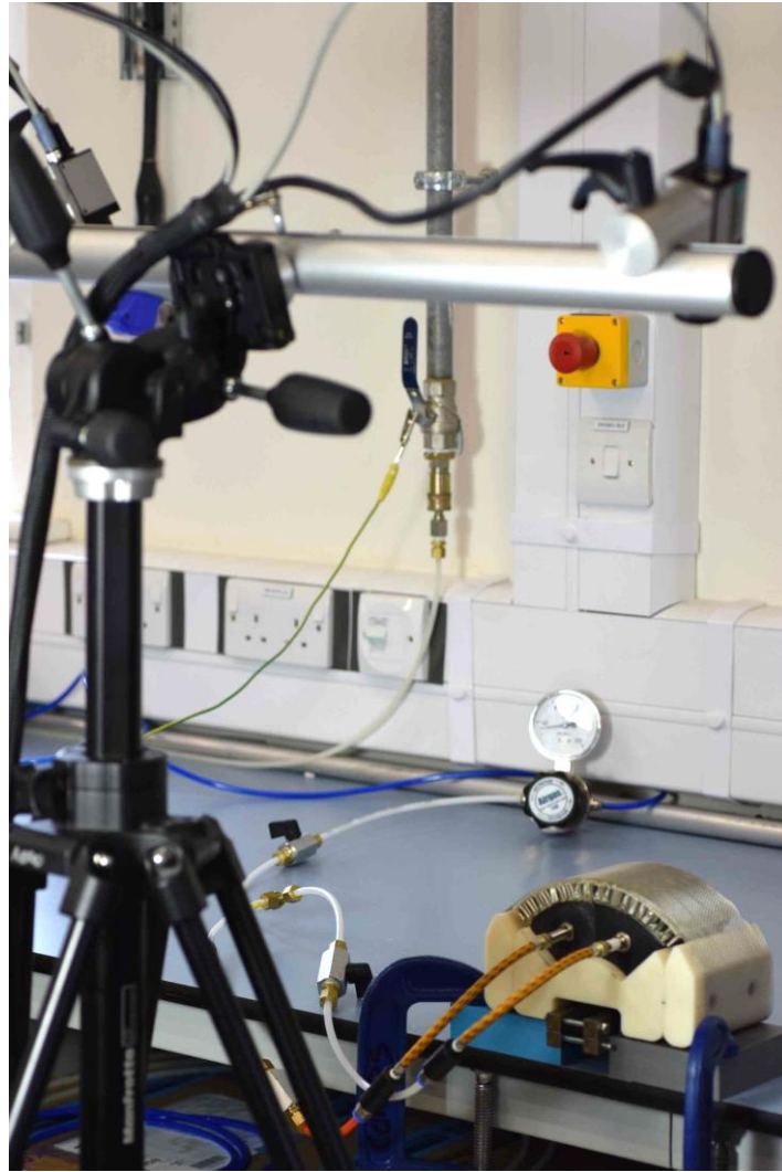
Figure 13. Test rig setup for 2-camera video gage system
