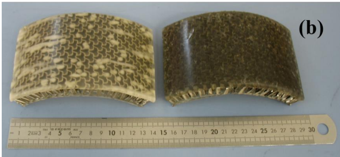
Figure 2. (a) Custom-made steel moulds of the upper and the lower face skins, filled with TPU pellets prior to compression moulding, (b) Flexible sandwich panels, left: with TPU skin, right: with graphene doped thermoplastic polyurethane (G/TPU) skin
