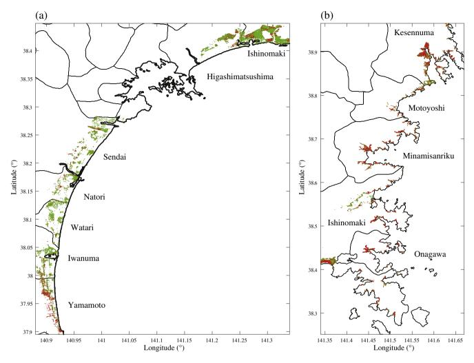
Fig. 16. Spatial representation of the importance of flow velocity in the vulnerability model for (a) plain-type coast and (b) ria-type coast.
