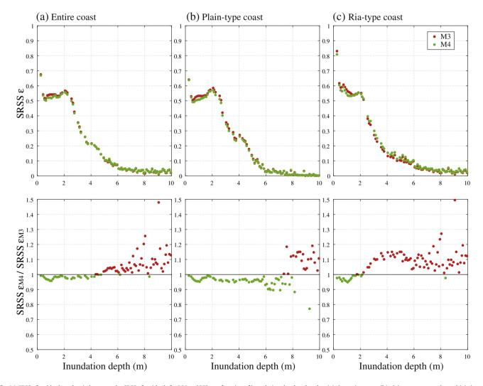
Fig. 14. SRSS of residuals and ratio between the SRSS of residuals for M4 and M3 as a function of inundation depth, related to (a) the entire coast, (b) plain-type coast only, and (c) ria-type coast only.
