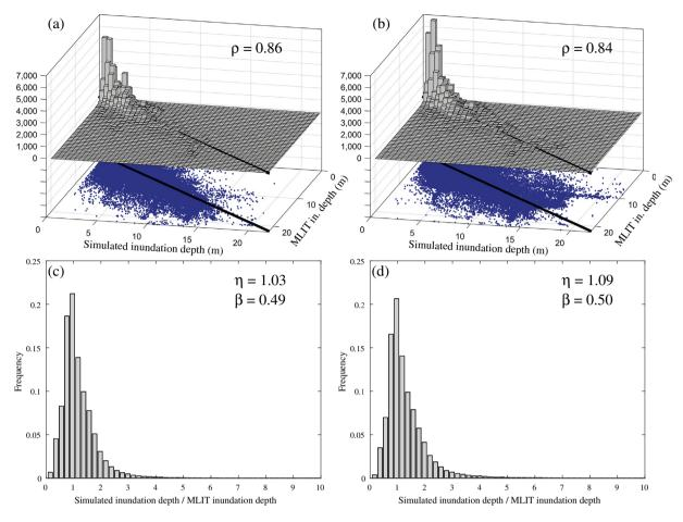
Fig. 4. Comparison of the MLIT and simulated inundation data based on the Satake et al. model: scatter plot and 3D histogram of the MLIT and simulated inundation depth data for (a) 10-m and (b) 50-m resolution, respectively, and histograms of the ratio between the MLIT and simulated inundation depth data for (c) 10-m and (d) 50-m resolution, respectively.
