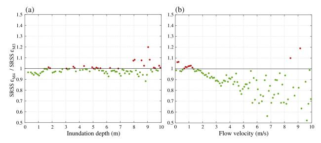
Fig. 18. Ratio between the SRSS of residuals for M4 and M3 as a function of the (a) inundation depth of (b) flow velocity for the models calibrated based on data for ria-type coast only.
