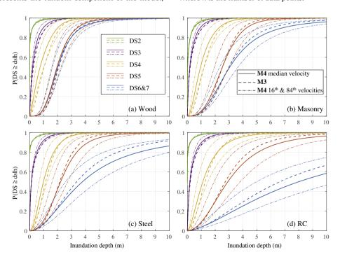
Fig. 8. Empirical fragility functions for four different structural typologies according to M3 (dashed lines) and M4 (solid lines for median velocity value, i.e. 1.84 m/s, and dashed-dotted lines for the 16th and 84th percentile velocity values, i.e. 1.00 m/s and 5.80 m/s, respectively).
