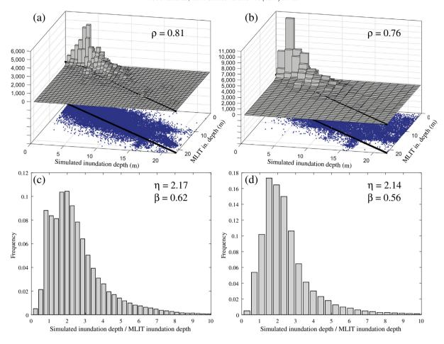
Fig. 5. Comparison of the MLIT and simulated inundation data based on the 10-m resolution DEM: scatter plot and 3D histogram of the MLIT and simulated inundation depth data based on the (a) Ammon et al. model and (b) linuma et al. model, respectively, and histograms of the ratio between the MLIT and simulated inundation depth data for the (c) Ammon et al. model and (d) linuma et al. model, respectively.
