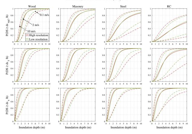
Fig. 10. Empirical fragility functions for four different structural typologies according to M4 considering a velocity of 0.1 m/s (dashed line), 2 m/s (solid line), and 10 m/s (dashed-dotted line), and using data from simulations at 10-m resolution (red line) and 50-m resolution (green line).
