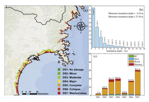
Fig. 1. (a) Spatial distribution of the MIIT damage data in Miyagi prefecture; (b) distribution of inundation depths; and (c) distribution of damage states for different structural typologies.
