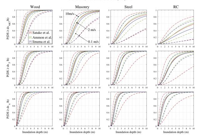
Fig. 11. Empirical fragility functions for four different structural typologies according to M4 considering a velocity of 0.1 m/s (dashed line), 2 m/s (solid line), and 10 m/s (dashed-dotted line), and using data from simulation at 10-m resolution according to the Satake et al. model (red line), Ammon et al. model (green line), and the linuma et al. model (blue line).
