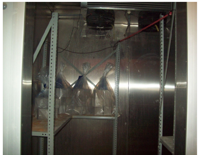
Figure 4. Test cubes under winter curing environment (C2).
