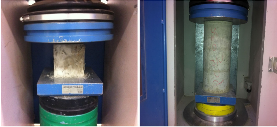
Figure 6. Compressive strength test using Avery Denison 2500 kN machines.
