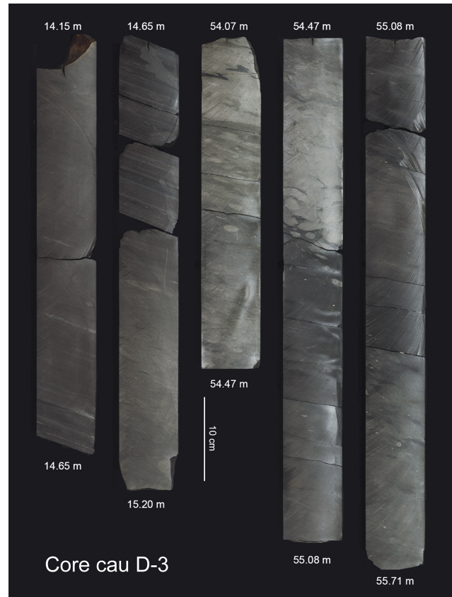
Figure 5. Massive and laminated, lightly bioturbated, facies of D-3 core between 14.15 and 15.20 m depth, and bioturbated facies of D-3 core between 54.07 and 55.71 m.
