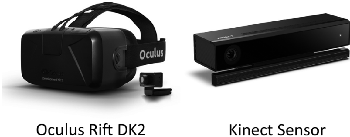
Figure 1. Virtual Reality glasses (Oculus Rift DK2) and Depth sensor (Microsoft Kinect 2 sensor) are the devices required to perform the tests.
