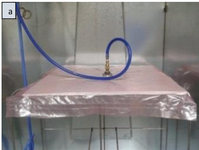
Figure 3. a) oven/vacuum curing of the plate b) curing cycle.
