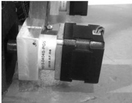
Fig. 9 NEMA 17 Motor with 5-to-1 gear ratio installed
