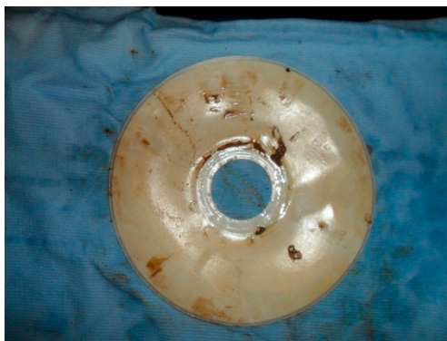
Figure 13. Impact of fouling on the rotating MBR system—even caking is observed.
