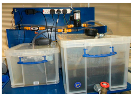
Figure 3. Static square-shaped membrane bioreactor (MBR) system in operation. The square membrane module is located in the larger tank on the right for filtration purposes.
