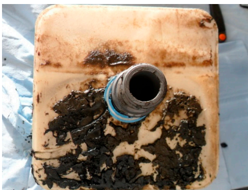
Figure 14. Impact of fouling on the square-shaped MBR system—uneven caking is observed.
