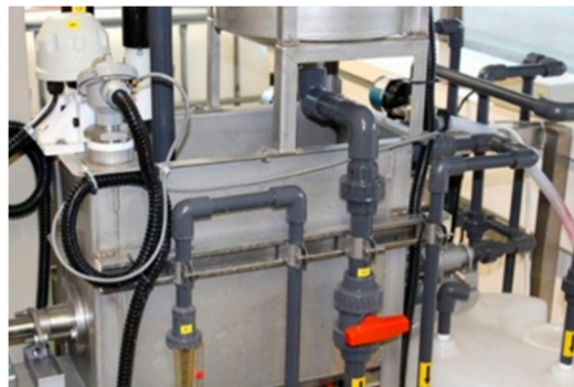
Figure 2. Rotating membrane bioreactor (MBR) system RPU-185 in operation. The membrane module is located in the batch tank for filtration purposes.
