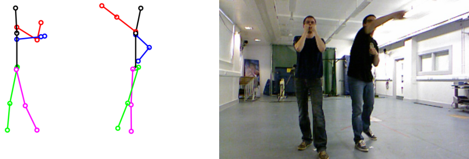
Figure 17 Example of a typical failure case caused by noisy skeleton data. The colour image (right) shows that this is a block interaction but our algorithm detects an attack interaction as the defend action is not correctly detected due to incorrect skeleton data for the player on the left. This instance will be penalised twice by the action point metric, firstly a FP for the attack and secondly a FN for the block.
