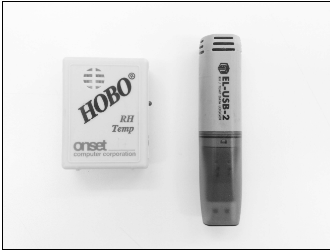
Figure 1: HOBO H8 and LASCAR EL-USB-2 dataloggers
