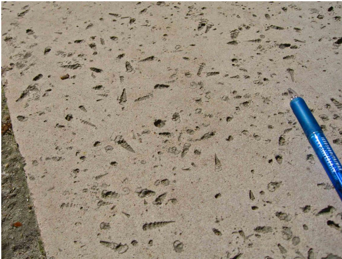
Fig. 11 : Lutetian limestone used for buildings: This example was used in the ‘Grand amphithéâtre’ of the Muséum National d’Histoire Naturelle in 1788. This rock is characterized by abundant moulds of gastropods (mainly ceriths) © P. De Wever
