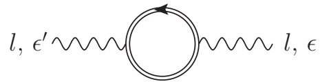
FIG. 2. The one-loop contribution to helicity or polarisation flip in a background field. The tree-level contribution is identically zero.
