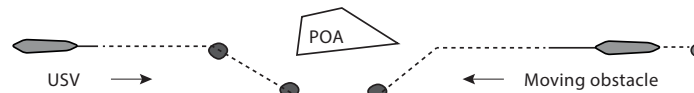
Fig. 1. The USV has to avoid the obstacle coming ahead passing port-to-port its projected obstacle area.
