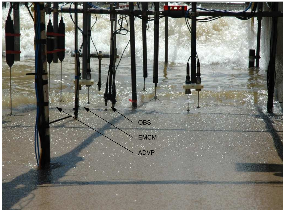
Figure 2: Picture of the relevant instrumentation on the swash scaffold rig. The arrows indicate the sensors used in this work: ADVP, EMCM and OBS. The CCP are buried and are not visible here.
