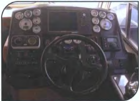
CNC-cut Carbon fibre panel (manufactured off-site): allows for rapid and accurate installation of gauges and instruments.
