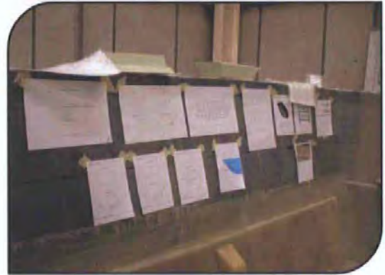
Drawings in use on shop-floor: promoting consistency in the manufacturing process and reducing the propensity for mistakes.
