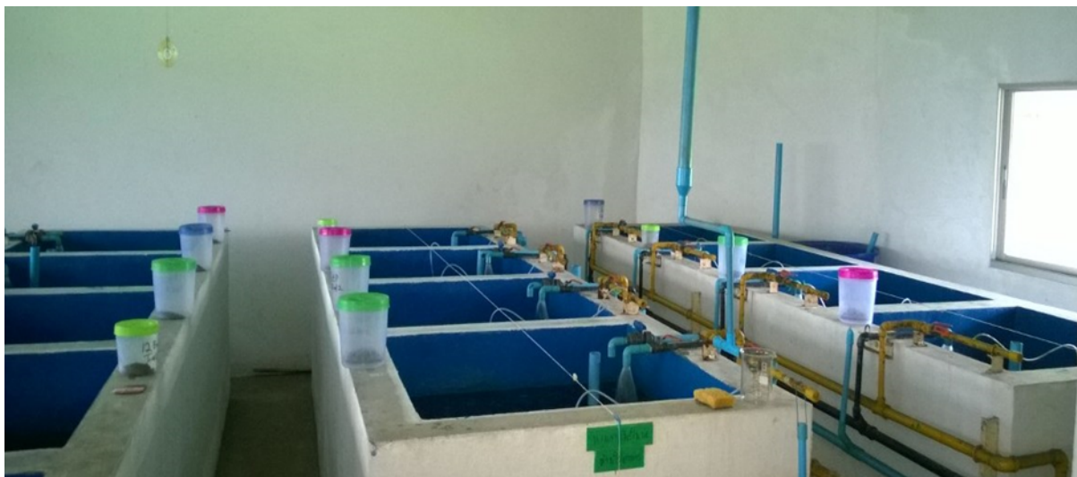
Figure 5.1: Flow-through system (FS) at the Division of Animal Production Technology and Fisheries, KMITL where tilapia were held during the trial. The experimental system consisted of square concrete tanks with a capacity of 508 L. Water was sourced from the local river system and was monitored daily (pH, DO and temperature) and weekly (nitrogen wastes – ammonia, nitrite, nitrate) to ensure appropriate conditions for tilapia.
