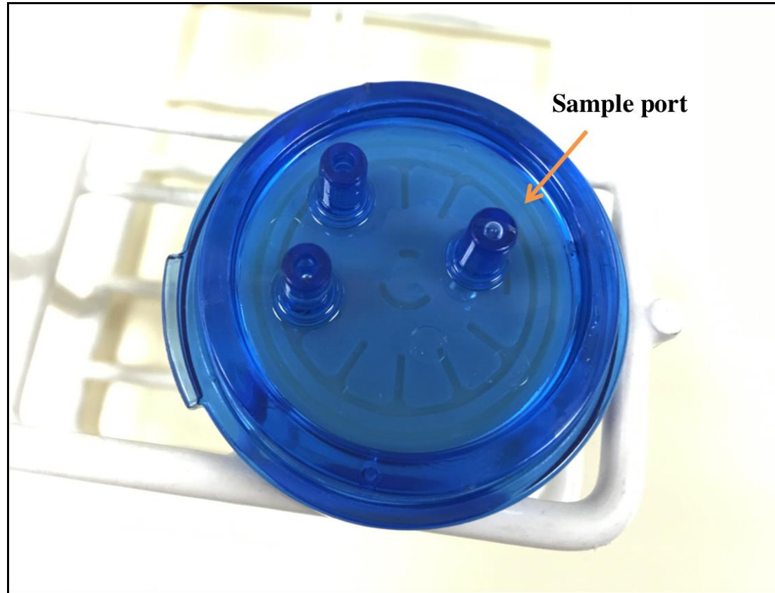
Figure 2.3 The sample port that was used to prepare the sequencing template for the clonal amplification.
