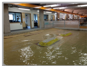
Long-crested waves encounter breakwaters in the Coastal Basin
