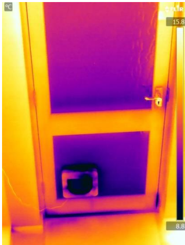
Figure 1. Example of a thermal image showing cold air coming into the home through a cat flap.
