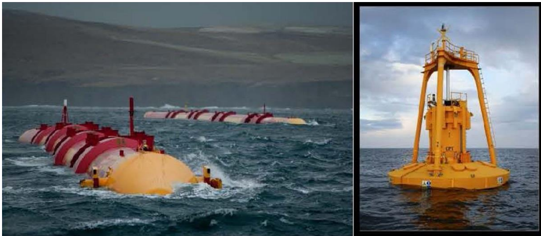
Figure 13: Examples of oscillating body converters: Pelamis II, left (courtesy of Pelamis Power, left [93]) and PowerBuoy, right (courtesy of the Ocean Power Technologies Inc, right [94])
