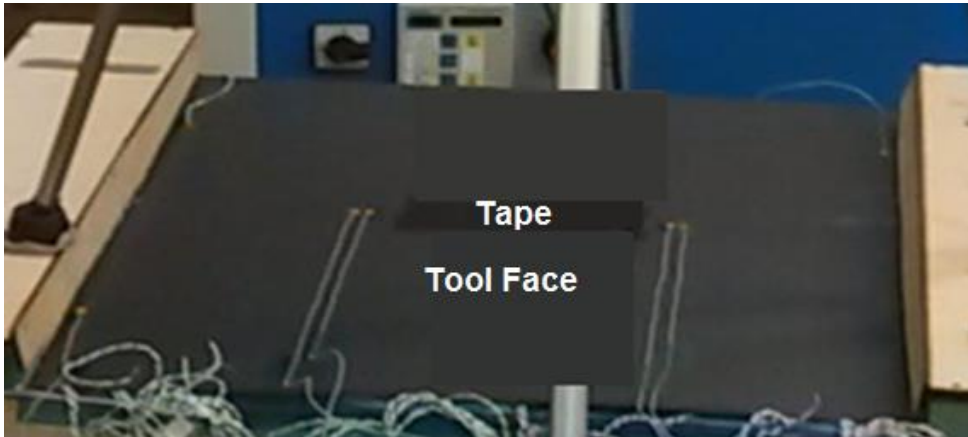
Figure 5-18 Black tape on the tool face as a reference for measuring emissivity.
