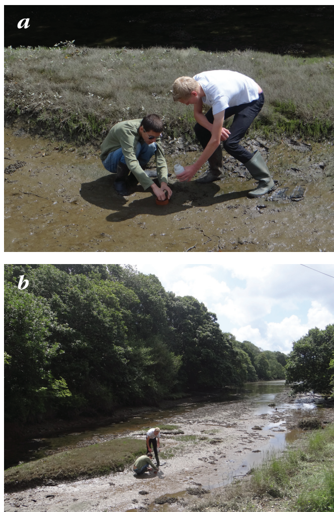
Figure 4. Collection of field samples at Trethem Mill at the tidal limit of the Percuil River. (a) Sample collection within the 10 cm diameter plastic ring. (b) Looking along the Percuil River, downstream towards St Mawes.
