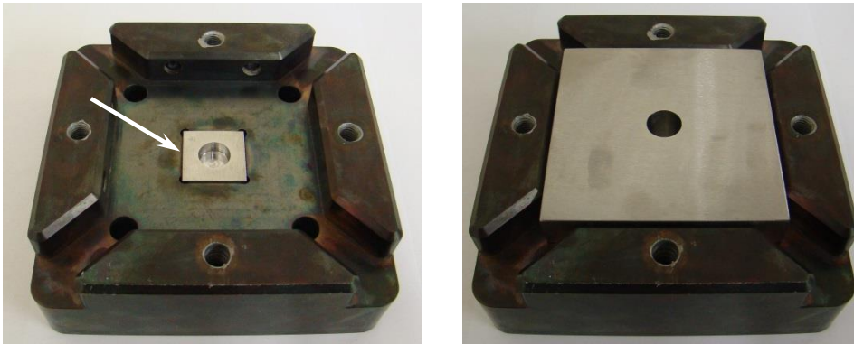
Figure 9 Illustration of a test piece used to simulate FHPP on damaged blade attachment fingers. The arrow indicates the backing plate in a recess in the bottom fixture.
