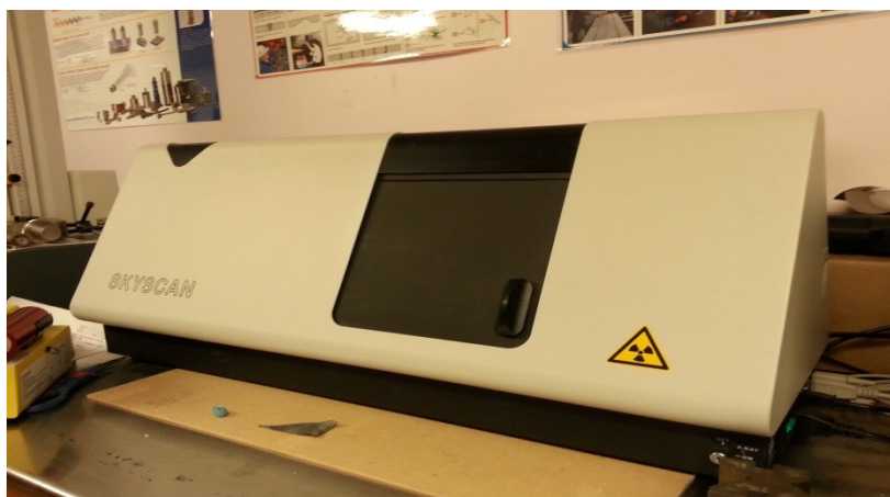
Figure B1-4: The X-ray tomograph (Micro CT) scanner for nondestructive three-dimensional microscopy.
