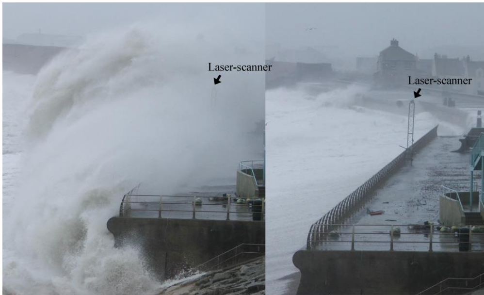
Figure 5.3 Sequence of photos showing the deployment of the laser-scanner on top of the seawall at Chesil on the 05/02/14 during an extreme storm.
