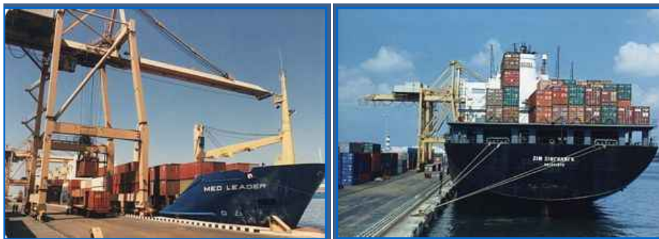
Figure 4.6: A close shot of Gantry Crane while handling ship containers at the quay (Source: ACCHC, 2009)
