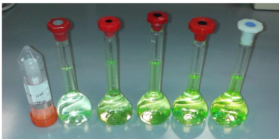
Figure 2.11: Fluorescein standards are yellow in colour. Here they increase in concentration from left to right ranging from 0 to 5 \text{ mg L}^{-1} .
