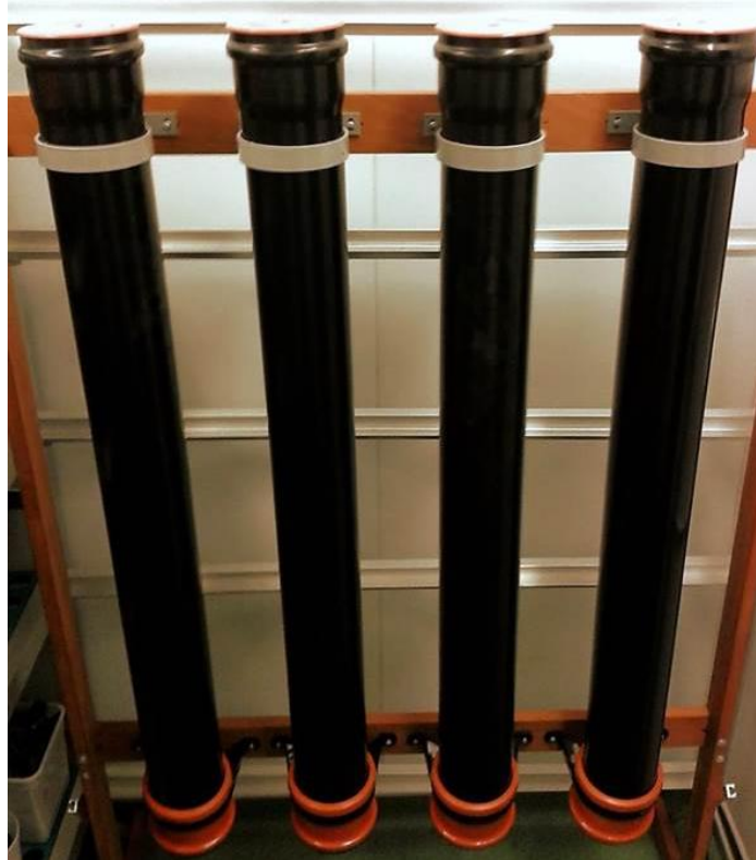
Figure 4.1 Soil column bioreactors used to assess the nutrient retention characteristics of Eden Project soils.
