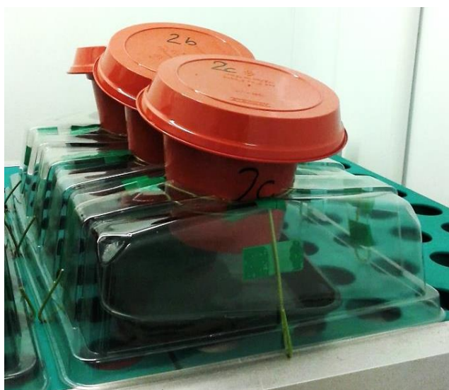
Figure 5.1: Replicate soil mesocosms used to measure the effect of biochar application on nutrient retention in artificial soils at the Eden Project.
