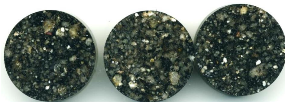
Figure 2.3: Polished resin sample blocks of freshly prepared artificial soil, analysed using the QEMSCAN ® instrument (Photograph courtesy of G.K.Rollinson, December 2013).
