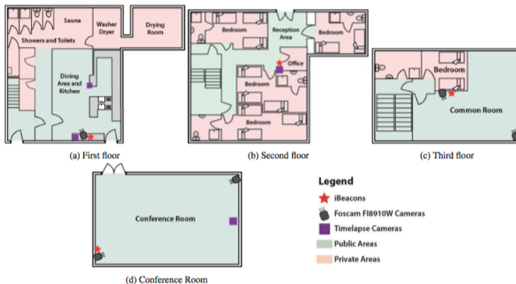
Figure 1: Hostel floor plan. Bedrooms were located on the second (b) and third (c) floor, and shared social spaces on the first (a) and third (c) floor. Areas marked green were recorded throughout the study; red areas were deemed “private”.
