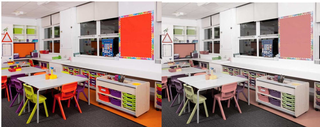
Figure 4 – (left) Strong colour contrasts in a primary school (Courtesy of EME Furniture, reproduced with permission); (right) same figure with contrasts reduced
