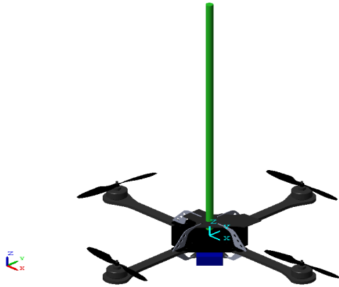
Figure 1. Fixed body and world coordinate systems.
