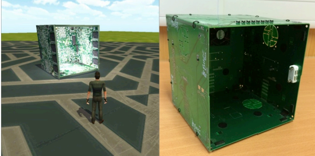
Figure 5. A desktop sized emulated intelligent environment (right) and its virtual representation (left).
