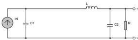
Appendix Figure 4.2: Bus Connected Buck Converter - ON
