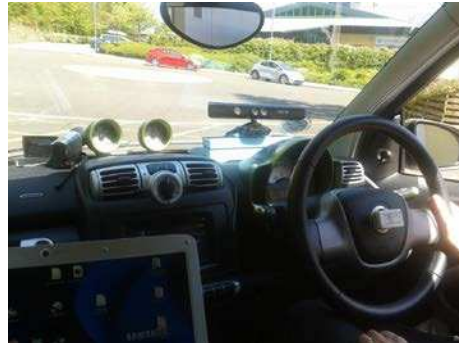
Figure 3: Kinect device and gyroscope inside a Smart Fortwo EV.
