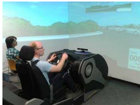
Figure 4: Kinect device and gyroscope in the driving simulator.
