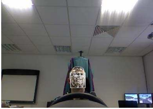
Figure 1: Face tracking achieved by the Kinect device in the Smart FortTwo EV and in the driving simulator.
