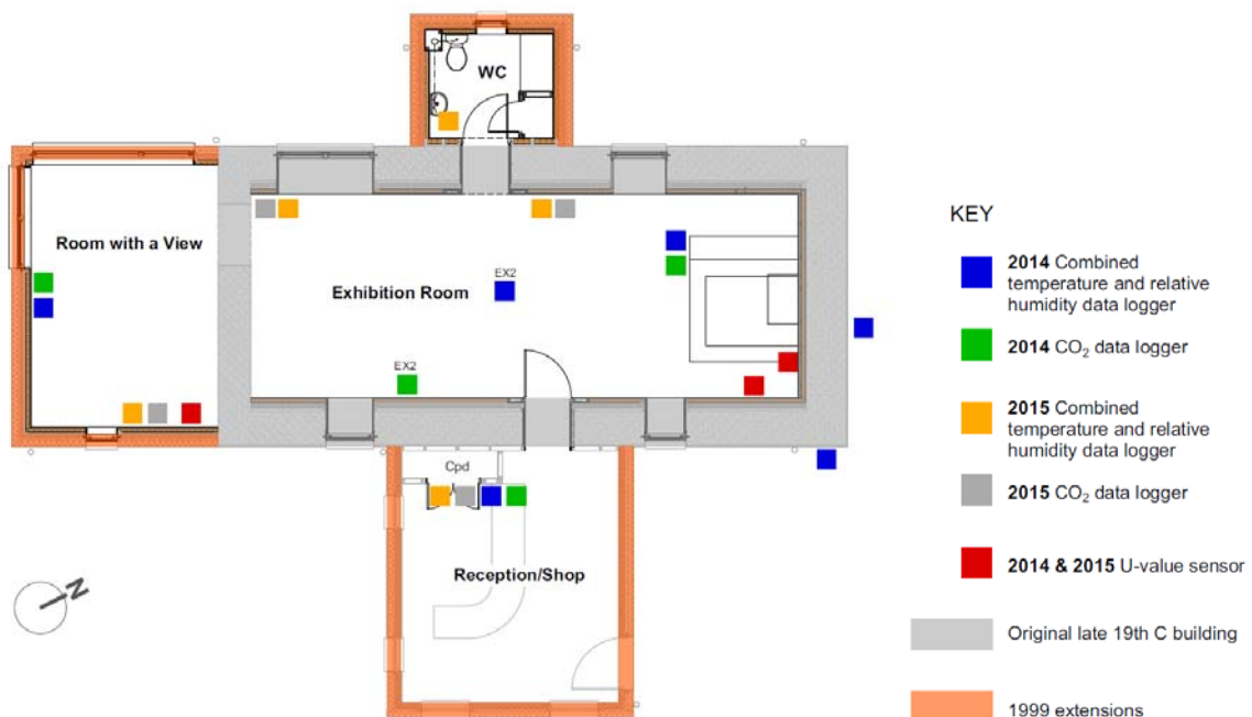
Figure 2. Plan view of LSIC building, indicating the historic core, 1999 extensions and location of monitoring apparatus for pre and post-refurbishment BPE.
