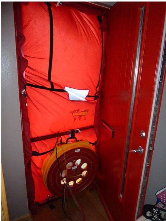
Figure 2. Airtightness testing (Source: MEARU)
