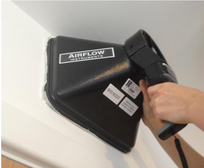
Figure 8. Testing of airflow rates (Source: Gráinne McGill)
