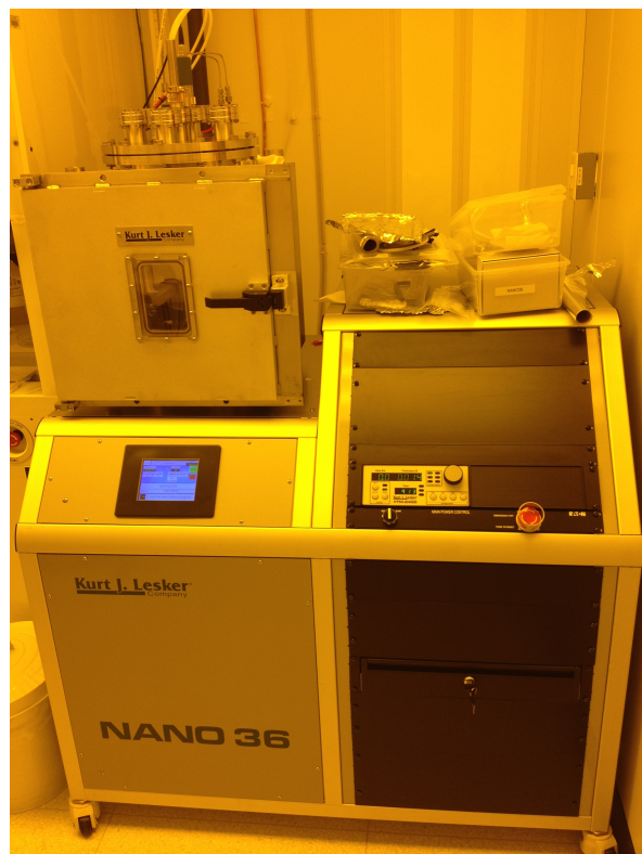
Figure 4.7: Nano36 is used to evaporate metal on the sample, it operates at a pressure of 10^{-7} torr, on the left a schematic representation of the machine.
