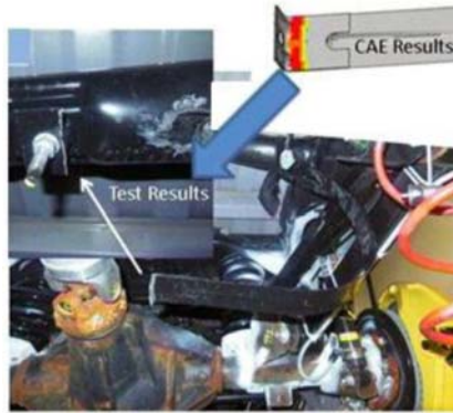
Figure 2-5 CAE correlation of rear strap fatigue [21]
