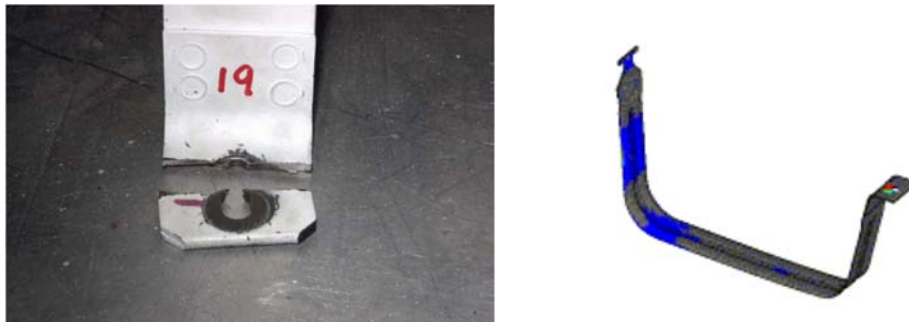
Figure 2-7 Sample #2, the rear strap cracked due to a loose strap and CAE fatigue prediction [22]
