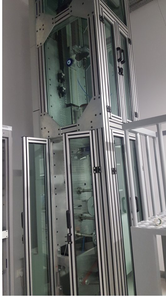
Figure 3.5: Fiber tower used for drawing fibers at low temperature below 800 degrees Celsius
