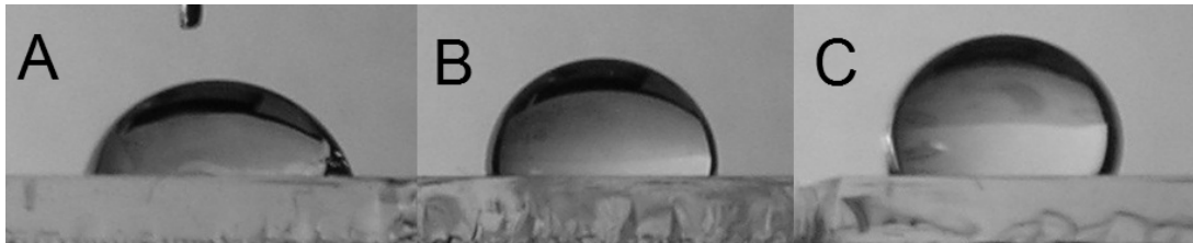
Fig.5. Water drop on the surface of PbSnS thin films (A) T_{sub}=268^{\circ}\text{C} , (B) T_{sub}=330^{\circ}\text{C} , (C) T_{sub}=361^{\circ}\text{C}
