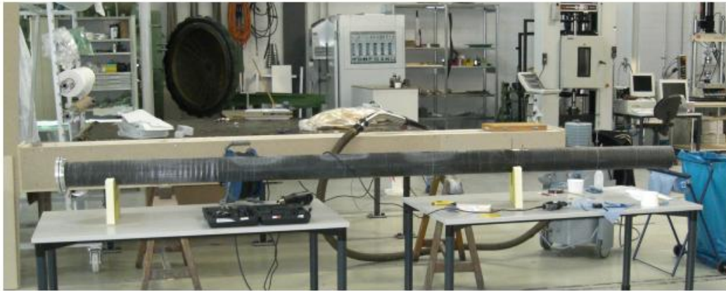
Figure 69. Boom after curing and removal of peel ply.
