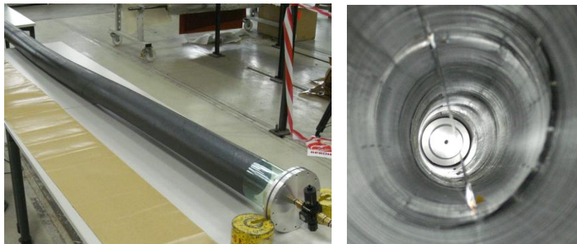
Figure 67. Breadboard of the deployable/inflatable boom with EAPs.
