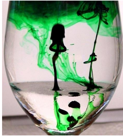
Fig. 1.1 (A) Buoyant plume of dyed alcohol rises through an interface between corn syrup and water (Copyright © Jessica Todd, College of Engineering, University of Colorado, Boulder, 2002. All rights reserved.) (B) Negative buoyancy experiment (Copyright © Cody Taylor and Gala Camacho, University of Colorado, Boulder, 2005. All rights reserved)
