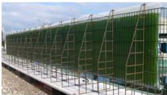
Fig.2.1.2.2. A) flat panel PBR. B) thin layer PBR.
